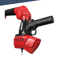
The Skyline scanner is an excellent solution for 3D analysis. High speed scanning and 200mm laser line allows you to detect the smallest details in record time. This scanner integrates into the handle with a quick detach features. No tools required.
