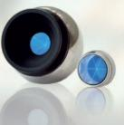
**Prismatic SMRs** use a solid glass prism that protects the reflective surface from dust. These types of SMR's are suited to outdoor environments where high dust concentrations can affect accuracy.
